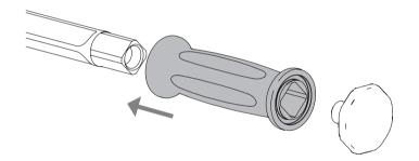
Once the Handle is secured, insert the Anvil; turn clockwise until secure.
