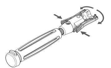
Pull the Impaction Head away from the Head Carrier then release the Arms.
