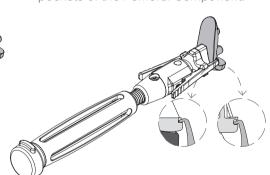
Visually check the Arms are located correctly within the Femoral Component as illustrated in the shown details. Pocket position may differ depending on implant design.
