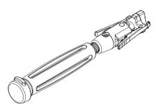
Visually check for any gaps between the Impaction Head and the Head Carrier to ensure the Impaction Head is fully seated.
