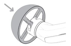
Twist in a clockwise direction to attach.
