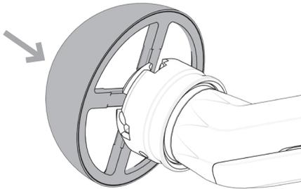
Twist the reamer in a clockwise direction to lock into the coupling.
