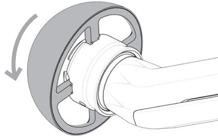
To detach, pull sleeve away from reamer and twist reamer anticlockwise to remove.
