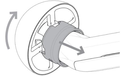
Note that if the drill is not attached you may need to hold the protruding end of the Offset Drive Shaft to prevent rotation of the coupling head.
