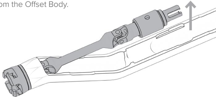
Pull the Offset Drive Train out of the distal end of the Offset Body.
