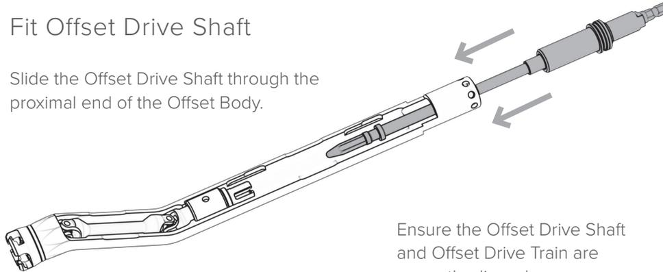
Ensure the Offset Drive Shaft and Offset Drive Train are correctly aligned.
