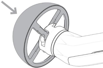
Twist in a clockwise direction to attach.
