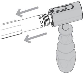
Ensure the handle securely locks into position by pushing it towards the Offset Body until you hear an audible click.
