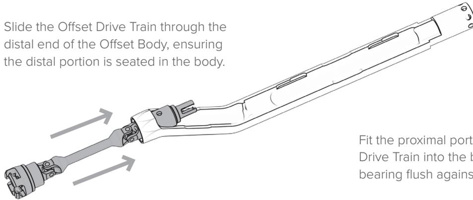
Fit the proximal portion of the Offset Drive Train into the body, pushing the bearing flush against the shoulder.
